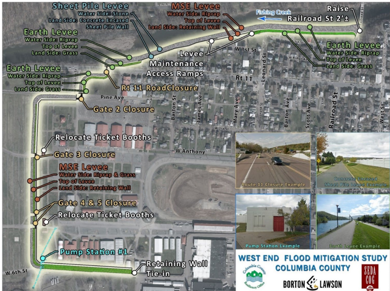
Figure 6.1 – Proposed Conditions Levee Alignment
